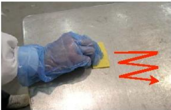
Figure 7.2. Hydrated sponge swabs are used to sample a process area surface.
